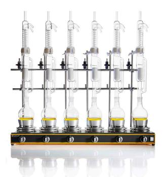
Apparatus for classic, manual extraction using the Soxhlet method.
