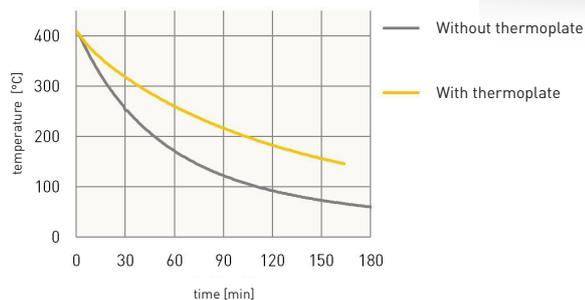
Comparison heat development block (thermoplate without fan)
