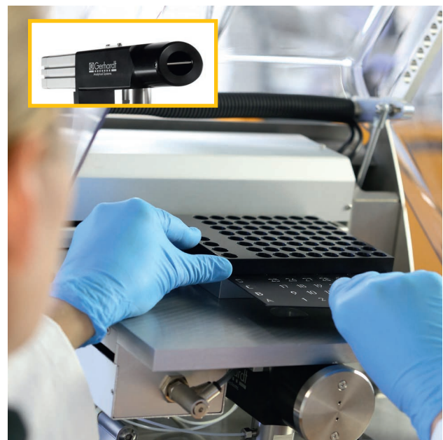
Figure 2: Autosampler with purge function - a purge chamber is continuously purged with helium before the sample is mechanically or manually fed to the combustion by the slider.
