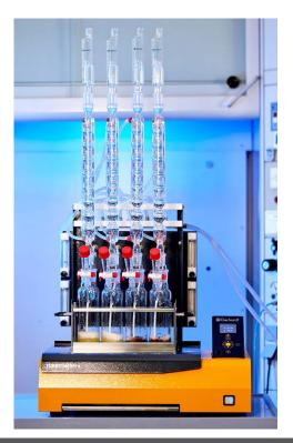
Digestion unit with infrared technology and modern control. Especially developed for boiling and distillation process with subsequent quantitative determination of sulphur dioxide content based on Monier-Williams method. Proven C. Gerhardt technology based on the TURBOTHERM TTs rapid digestion unit. Rapid and consistent heating by means of infrared technology.
