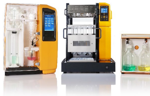
Fig. 9: Complete system for nitrogen analysis according to Kjeldahl, consisting of 20-unit KTL-20 digestion system (centre) with TURBOSOG gas scrubber (right) and VAPODEST 500 water steam distillation unit with implemented titration (left).
